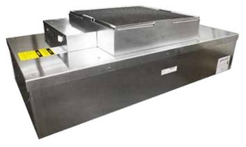
By taking advantage of a unique combination of EC motor technology coupled with Envirco's proprietary baffling system and backward inclined fan, the LE-DC leads the industry in energy-efficiency. Its electronically commutated (EC) motor with internal microprocessor offers high performance and delivers long motor life with energy consumption rates as low as 90W @ 90 fpm.
